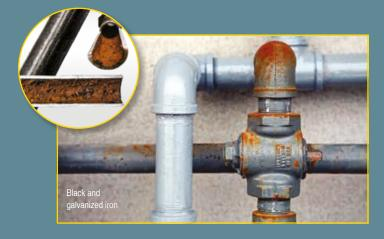
This actual cutaway of black iron compressed air piping shows typical contaminant build up and flow restriction after just a few years of operation.
