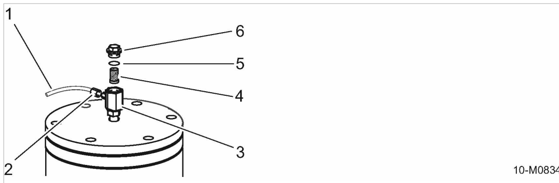
Fig. 38 Oil separator tank dirt trap maintenance
