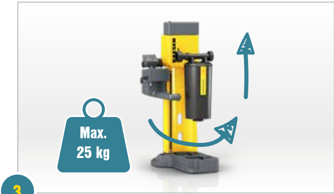
3 The cartridge is lifted out of the bayonet fitting with a 45° turn using its ergonomic handle. Fully saturated, it weighs a maximum of 25 kg.
