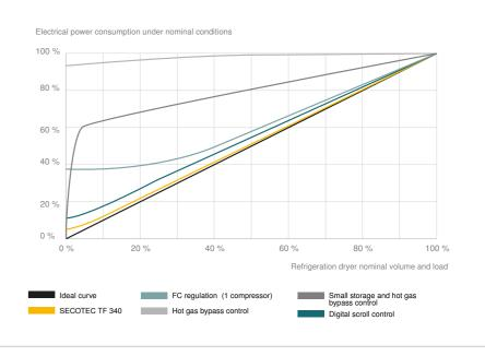
This means compressed air can be dried effectively even during start-up phases. The high-quality insulation around the thermal mass also helps keep energy use to a minimum. Compressed air drying with **SECOTEC** refrigeration dryers not only ensures exceptional energy efficiency, but also, thanks to their impressive thermal capacity, provides material-friendly operation.
