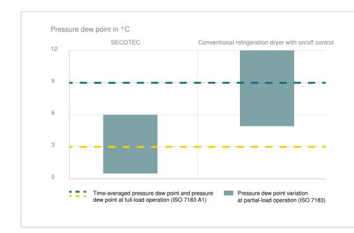
**SECOTEC** refrigeration dryers, on the other hand, ensure material-friendly operation thanks to their high thermal mass storage capacity. Once the thermal mass has been charged, the refrigerant compressor and fan motor can remain switched off for much longer with no impact on pressure dew point stability.
