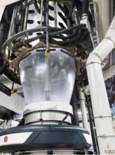
Image, left: Huge sheets of foil are produced inside these towering extruders.
