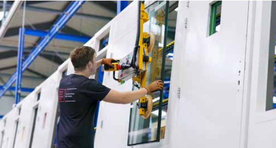
Doors, windows and frames are fully glazed and finished on site.
