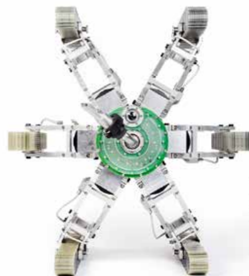
The JETTY robot, created in partnership with the Faculty of Electrical Engineering at the Technical University of Prague, is used for large installations and particularly heavy contamination.
