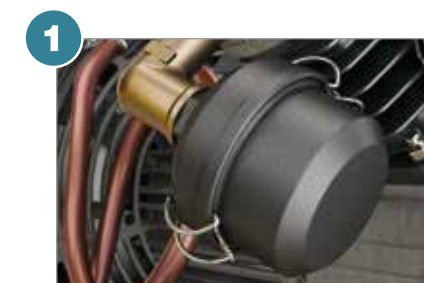
Silenced air intake filter
