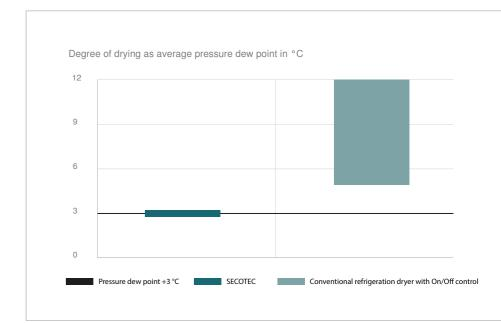
SECOTEC refrigeration dryers, on the other hand, ensure material-friendly operation thanks to their high thermal mass storage capacity. Once the thermal mass has been charged, the refrigerant compressor and fan motor can remain switched off for much longer with no impact on pressure dew point stability.
