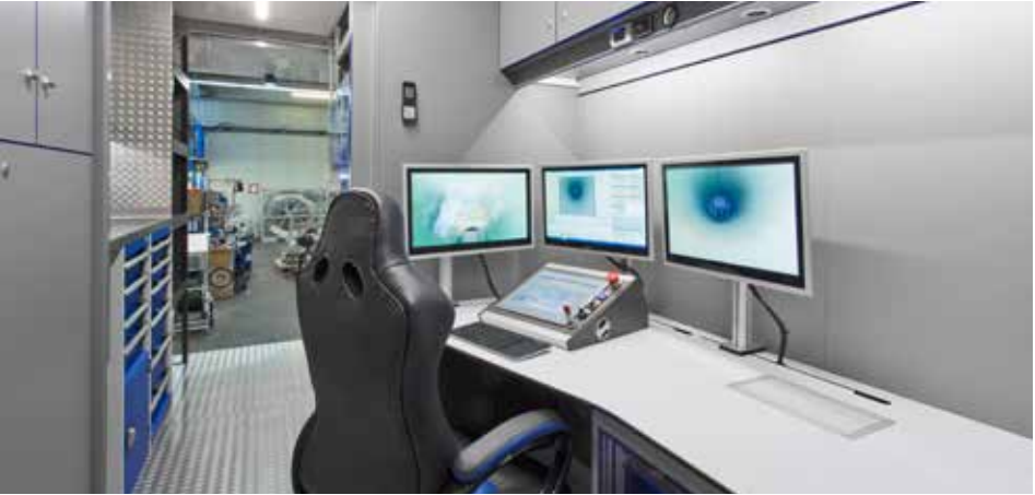
Image above: The high-end, self-contained rehabilitation vehicles carry all the equipment required for the innovative UV liner method. Image below: An interior view of the specialised rehabilitation vehicle.
