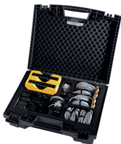
Figure 2: Measuring equipment for an Air Demand Analysis.
