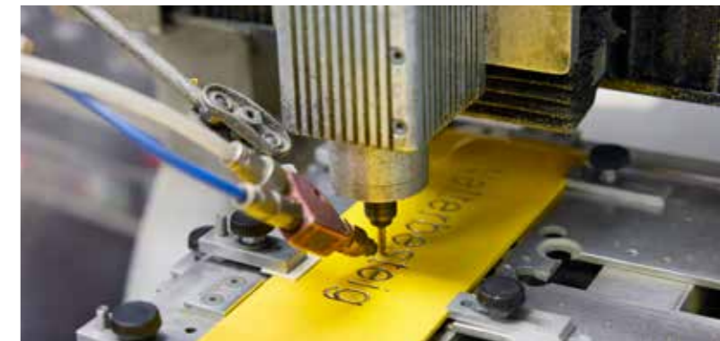
Compressed air is used at almost every production workstation: Laser-etching of table knives, cable manufacture, hose cutting, engraving (advertising technology).
